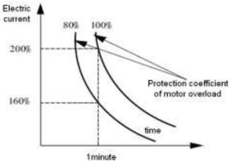
Picture Pa-2 Schematic diagram of motor overload protection coefficient
