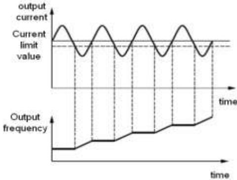
Picture PA-4 Current limit Schematic diagram of speed increasing
