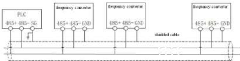
Fig. 3-6 Recommended wiring method for PLC/frequency converter multi-computer communication
