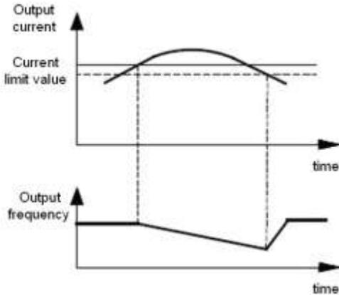
Picture PA-5 Current limit Schematic diagram of constant speed
