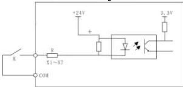
Fig. 3-7 Multifunction input terminal wiring
