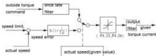
DIAGRAM P4-4 TORQUE CONTROL SIMPLIFIED DIAGRAM
