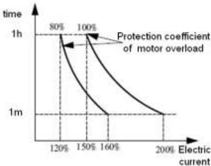
Picture PA-1 Curve of motor overload protection
