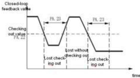
Picture PA-7 Checking out time of Closed-loop feedback lost
