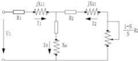
DIAGRAM P3-1 asynchronous motor steady state equivalent circuit diagram
