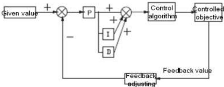
P8-2 PID adjusting schematic diagram
