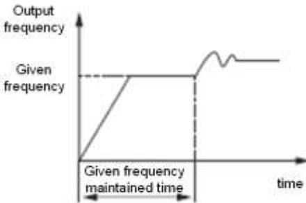
P8-6 closed cycle presetting frequency running figure
