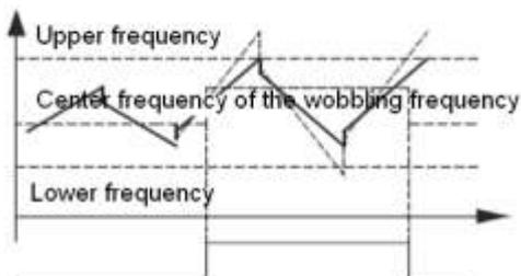
Picture p7-6 Schematic diagram of the limit of the range of wobbling frequency
