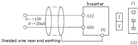
Fig. 3-3 Analog input terminal wiring diagram
