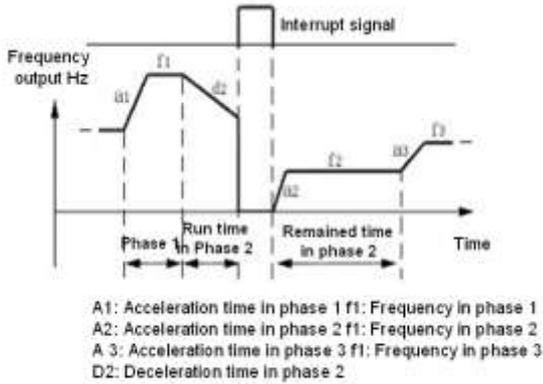
Figure P9-5 PLC Start mode 2
