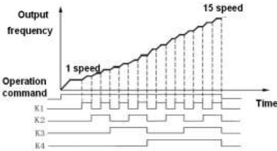
Chart P7-1 schematic diagram of multistage speed operation
