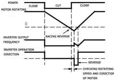
DIAGRAM P2-1 ROTATING SPEED TRACKING DIAGRAM
