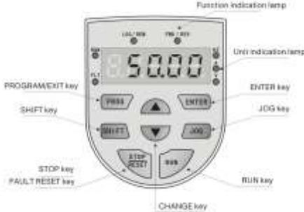
Fig. 4-1 SY7000 operation panel deployment diagram
