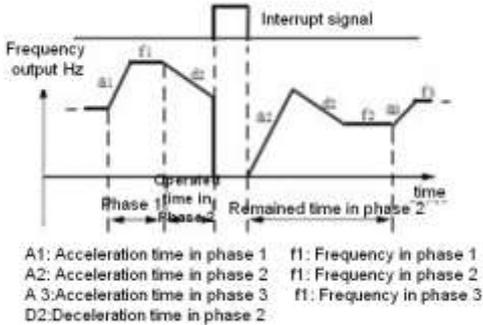
Figure P9-4 PLC Start model
