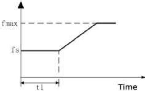
DIAGRAM P2-2 Starting frequency diagram
