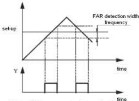
Picture p7-7 Frequency arrival schematic diagram
