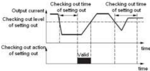
Picture PA-6checking out schematic diagram of setting out
