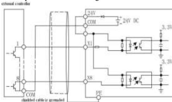
Fig.3-8 Source connection of using frequency converter's internal +24 power
