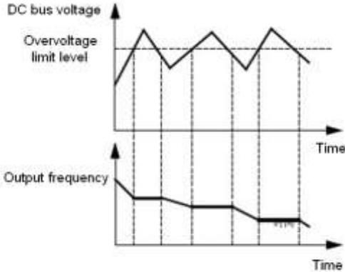
Picture PA-3 introduction schematic diagram of overvoltage limit level
