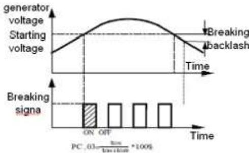
Picture PC-1 breaking diagram
