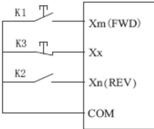
Picture p7-5 three-line control mode2 schematic diagram
