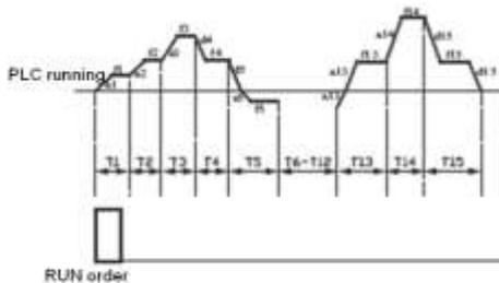
P9-2PLC diagrammatic sketch (maintain after a single-running process-)
