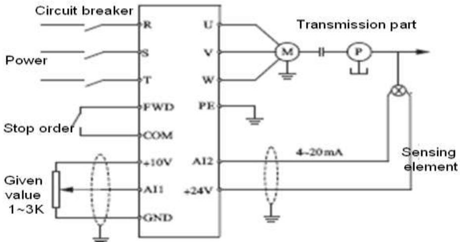
P8-1 simulate feedback control system schematic diagram
