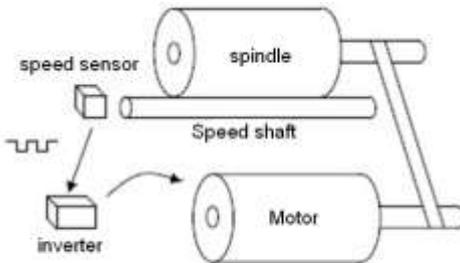
Picture P9-7 long time stopping function example
