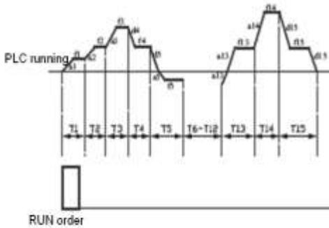
P9-1 PLC diagrammatic sketch (stop after a single-running process-)
