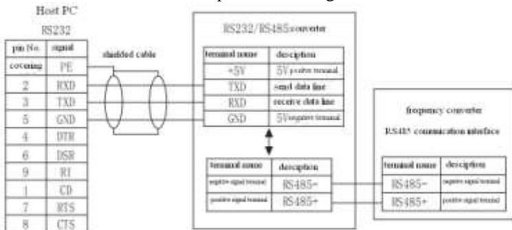
Fig. 3-5 Host PC and frequency converter interface and cable connection diagram
